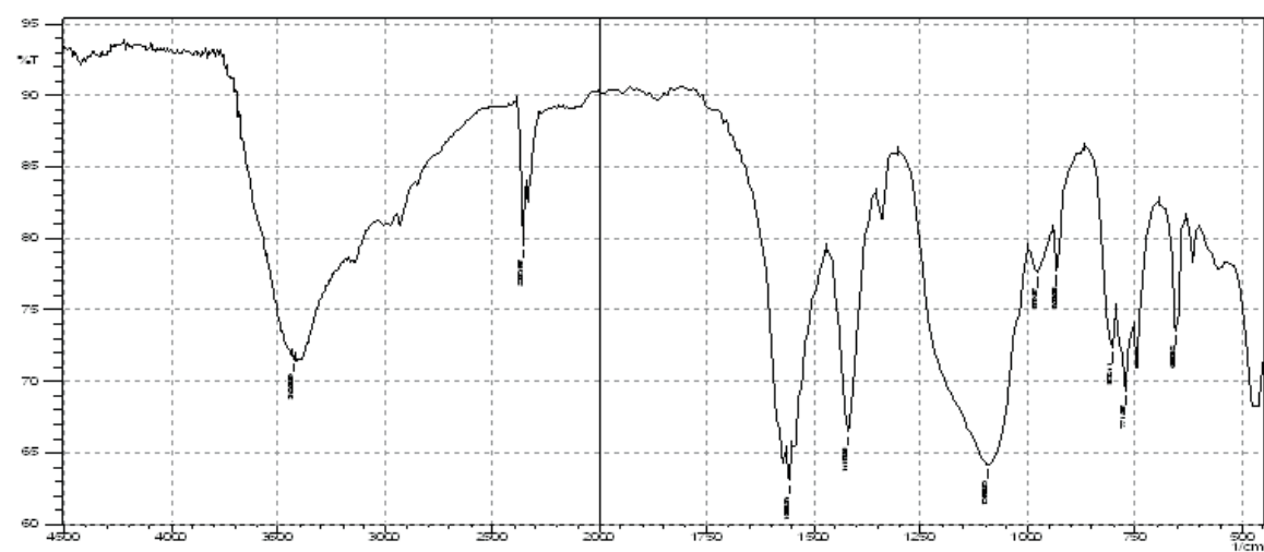
Fig.2 IR spectra of barium iodide
