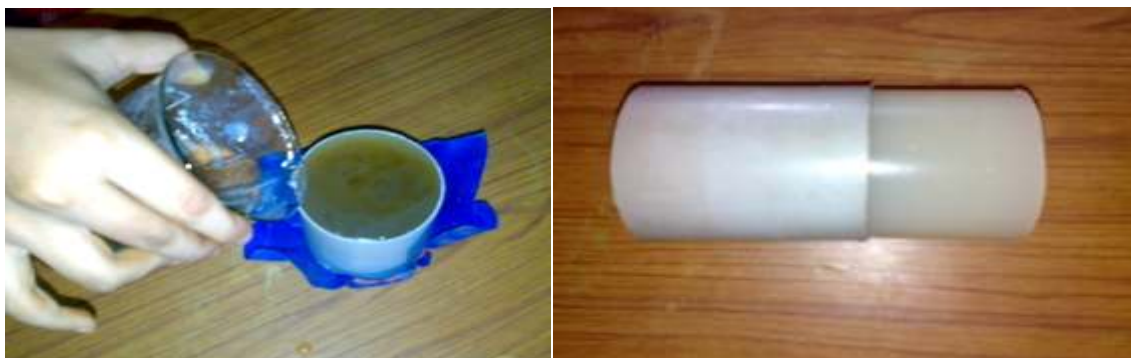
Figure 2 Preparation of the salt bridge
