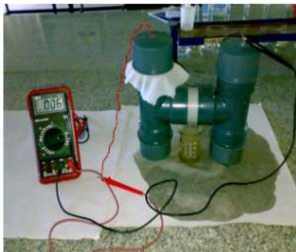
Figure 3 Setup of MFC and voltage fluctuation in the multimeter after 30minutes of stabilization
