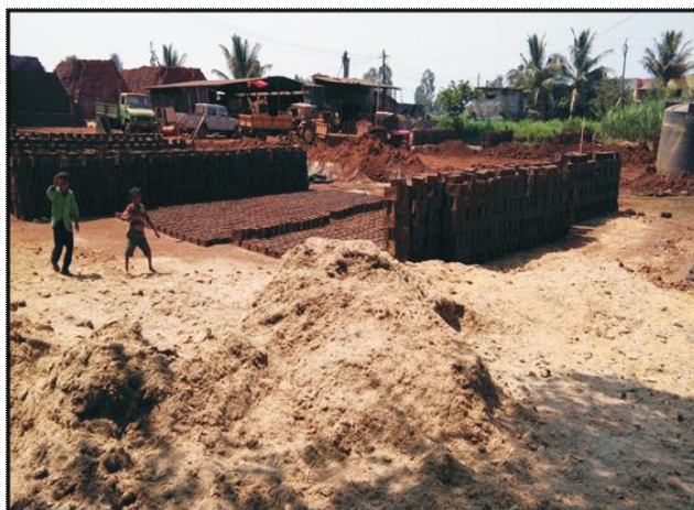
Photo plate 4 : Bagasse dust is used in manufacture of soil bricks.
