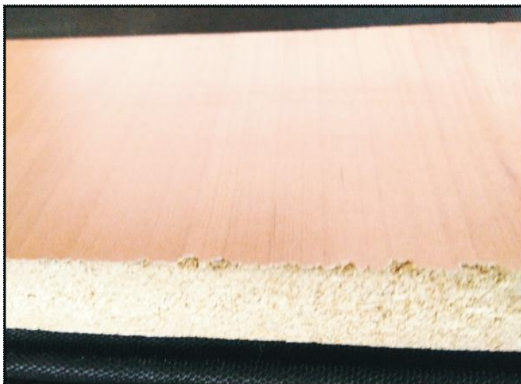
Photo plate 6 : Use of bagasse in manufacture of partical boards.
