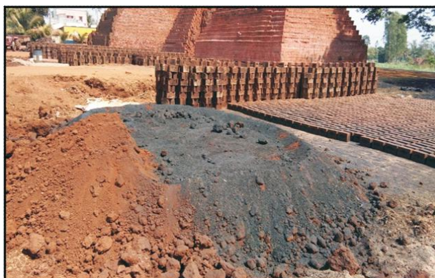
Photo plate 7 : Bagasse Ash is used in manufacture of soil bricks.
