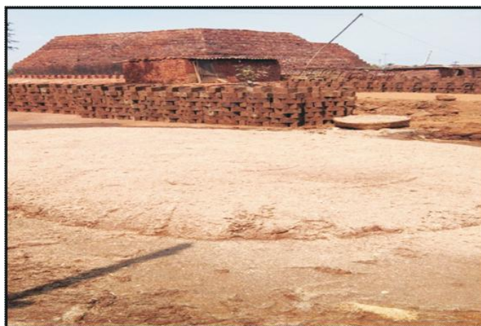
Photo plate 5: Bagasse dust is mixed with soil mud for manufacture of soil bricks.
